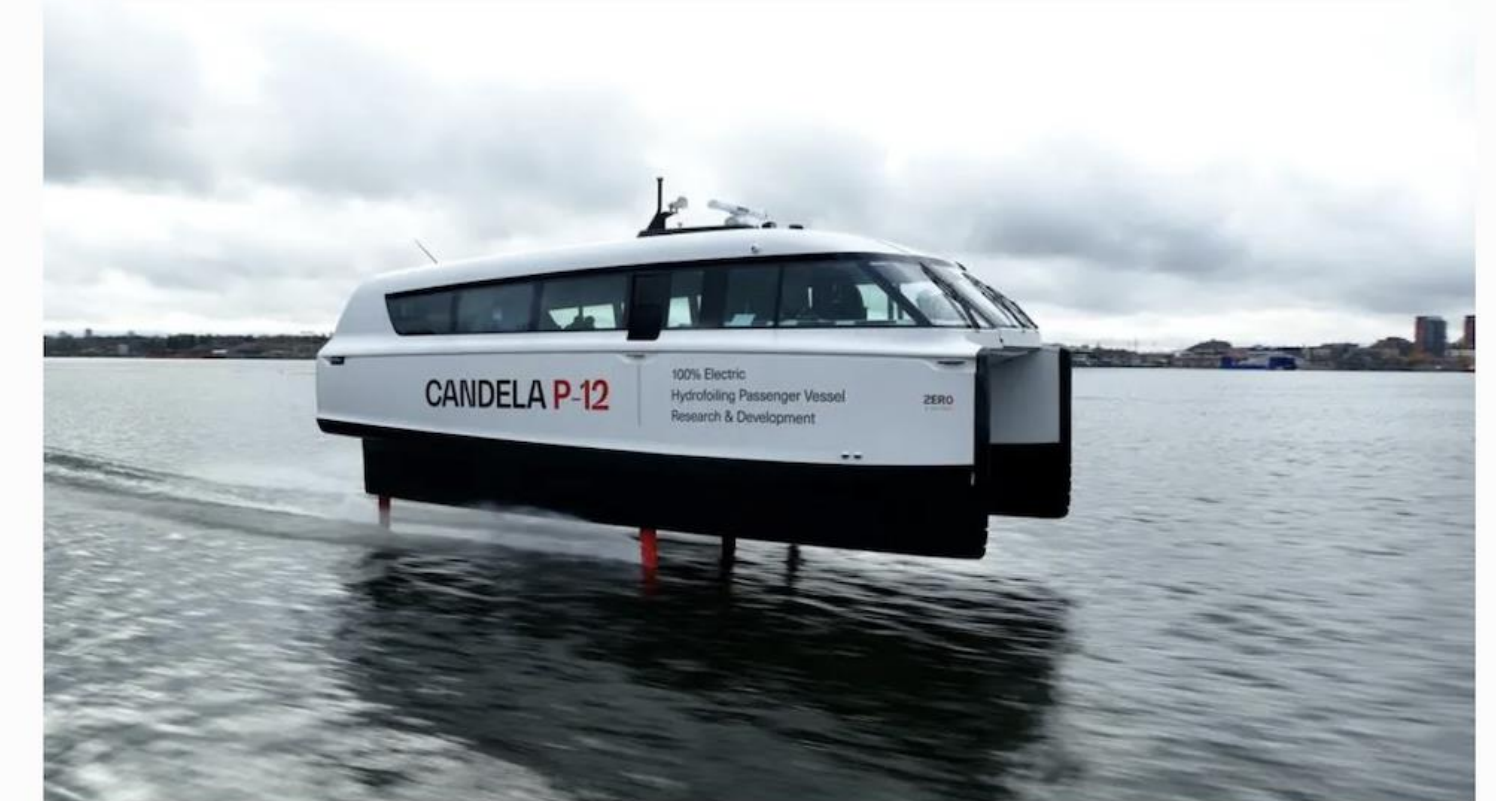
The all-electric-powered Candela P-12 ferry flies over the water on hydrofoils. CANDELA
